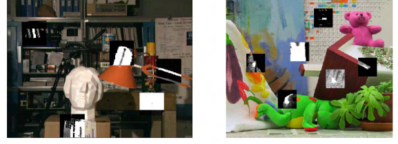
Fig. 3: Support window weight computation on Tsukuba (left ) and Teddy (right) images. The weights are computed not only on the active region ( which is pure white) but also on outside of this region therefore it can cover many variations of intensity value
