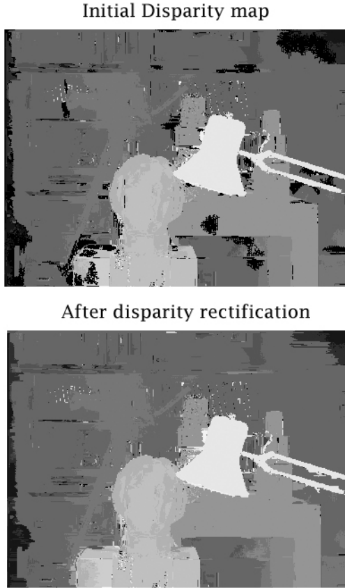
Fig. 4: Shows the initial disparity map computed by the first stage of algorithm and its corresponding output after the disparity rectification process
