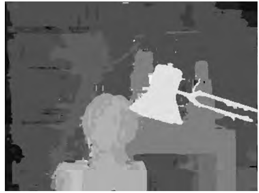
Fig. 5: Noise removal by the Median filter with 3x3 support size on the final output of the algorithm shown in Figure 4
